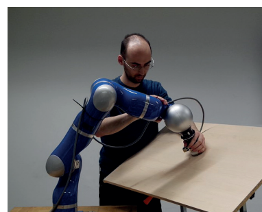
Figure 1: Demonstration of a circular wiping trajectory on a flat surface. The demonstrations were repeated for multiple orientations.
