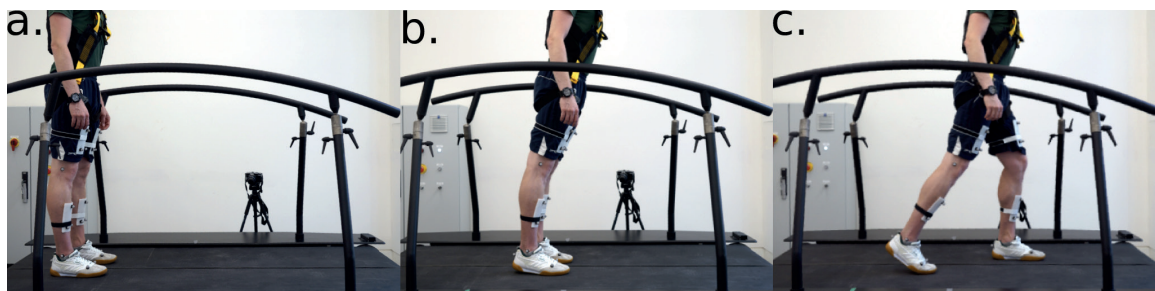
Figure 1: Time sequence of one experiment trial. (a) Participant in the start position facing forwards; (b) to the centre of the treadmill, where the belt stops and they begin to fall; (c) The subject takes a step to recover from the fall.
